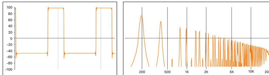
The square wave can be reshaped to make the waveform cycles, or pulses, more rectangular, by using a *pulse width modulation (PWM)* control. The more rectangular the wave becomes, the more nasal it sounds. When modulated in this way, the square wave is known as a *pulse wave*, and contains fewer harmonics. It can be used for reeds, basses, and brass sounds.
