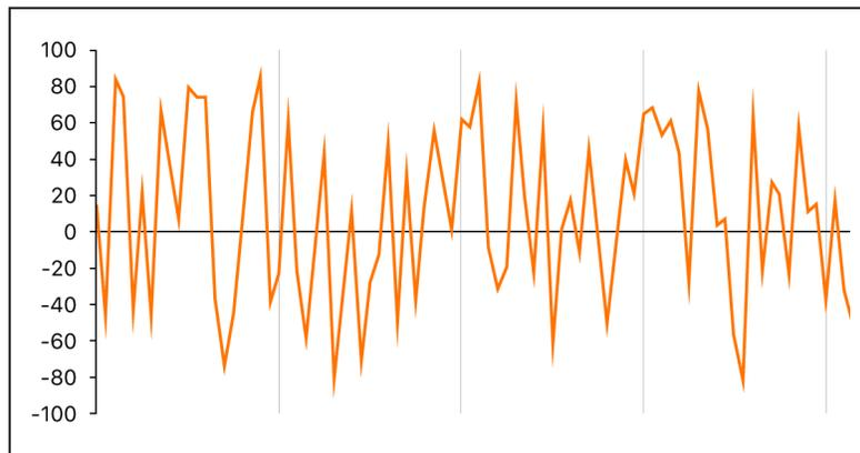
A repetition of a waveform—each peak and trough in the oscillogram—is known as a *cycle*. The number of cycles that occur per second determines the basic pitch of the waveform—commonly known as the *frequency*. Most instruments provide an oscillator frequency control, measured in hertz (Hz), that determines the number of cycles per second—and therefore the basic pitch of your sound.
