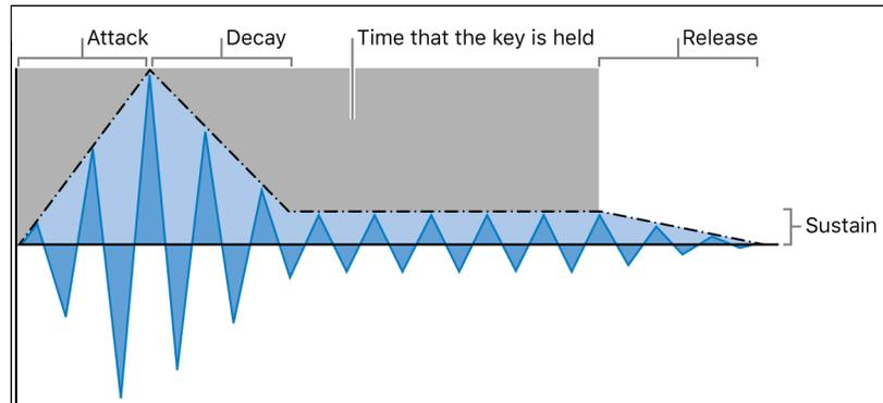
The envelope generator usually features four controls—Attack, Decay, Sustain, and Release, commonly abbreviated as *ADSR*.
