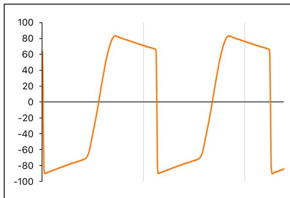
The figure shows an unfiltered sawtooth wave, with drive set to a value of 80%. Note the wave cycles touching the floor and ceiling of the filter dynamic range.
