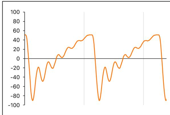
This resonant filter setting results in much brighter and harsher signals close to the cutoff frequency. Frequencies below the cutoff point are not affected.
