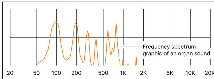
The illustration shows the level and frequency relationships between the fundamental tone and the harmonics at a particular moment in time. These relationships constantly change over time, which results in continuous changes to the frequency spectrum and, therefore, changes to the sound.
